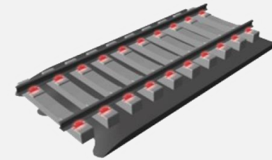
Continually supported slab (e.g. IVES)
