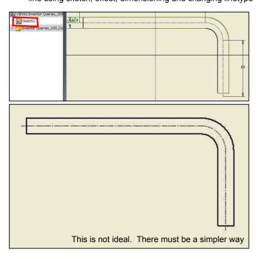
The other work around I have found is to retrieve the model sketch of the path for the sweep, and change the properties of the line to chain. You however don't get the extension beyond the edges in this case
