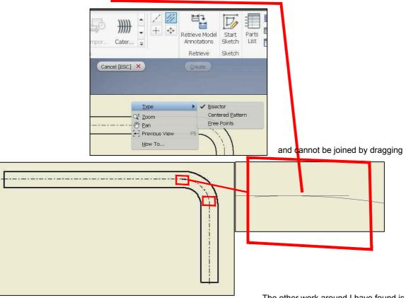
The work around I have found is to create the continuous centre line using sketch, offset, dimensioning and changing linetype
