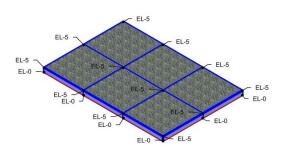
In this image you see the Depth Surface. For the purposes of this handout it will be called the Top of Pavement Section Surface. This surface is used to represent the materials actual depth.
