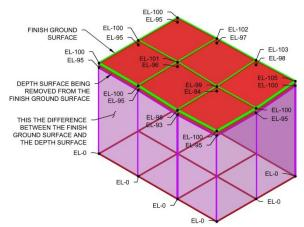
In this image you see how the Depth Surface (Top of Pavement Section Surface) is removed from the Finish Ground Surface during the creation of the TIN Volume (Composite) Surface.
