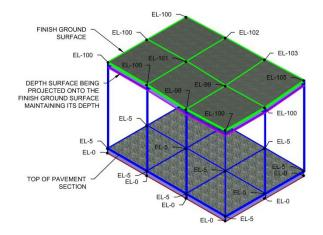
In this image you see the Depth Surface (Top of Pavement Section Surface) being projected up to the Finish Ground Surface with the use of a TIN Volume (Composite) Surface. Note: During the projection notice how the Depth Surface maintains it depth relationship, which in this example it 5, but it can vary if needed.
