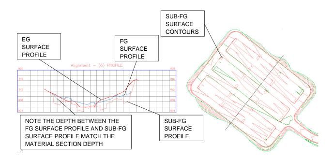
Note: The final surface in this scenario is what I term semi-dynamic. This is because if a section area changes in either its extents or depth, all you have to do is adjust the 3D object created in Step 2. Then it is just a matter of rebuilding the surfaces (if the Automatic Rebuild, is not set "On" for each of the surfaces). This is also true if the existing ground changes.
