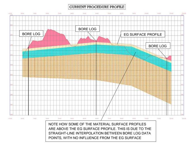
Note: The final surface in this scenario is what I term semi-dynamic. This is because if you have more bore log data to add you can add it to the surface created in Step 2 named "DEPTH-(material type)". Then it is just a matter of rebuilding the surfaces (if the Automatic Rebuild, is not set "on" for each of the surfaces). If the Existing Ground Surface changes it is just a matter of rebuilding the surfaces.
