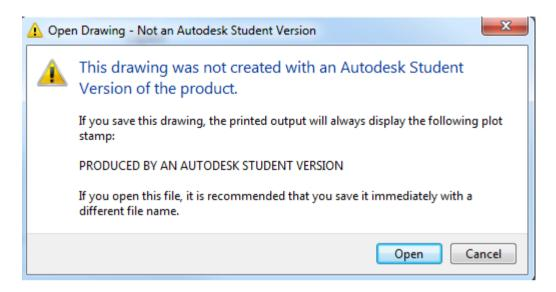
When using a commercial license of AutoCAD to open a drawing that was created using a version AutoCAD 2019 that displays the education watermark, the following task dialog is displayed:
