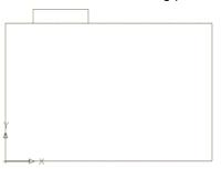
10. From the solids tab, select the pulldown under the Box tool, and select the *cylinder* tool. Place the start point using a *midpoint* snap along the bottom edge of the front face of the model:
