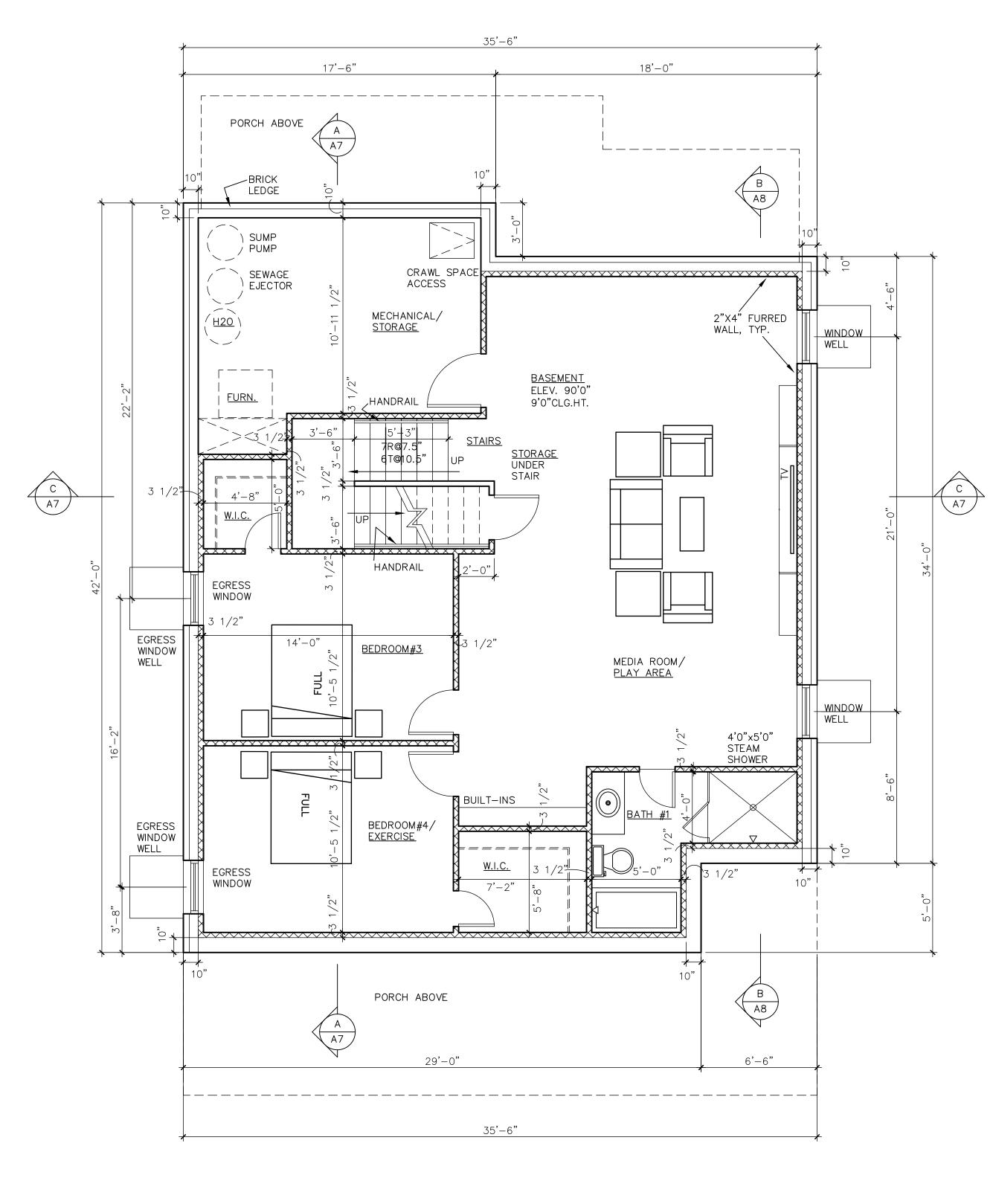
BASEMENT FLOOR PLAN SCALE: 1/4" = 1'-0"1,405 S.F.
