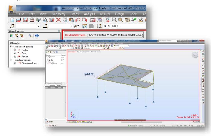
You can also switch between model types from the file menu: **Analysis > DAM Analysis > Main Model or DAM model.**
