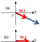
**In one active direction only** – notional loads created will act in the closest global axis direction of the resultant of all lateral loads in each load combination.
