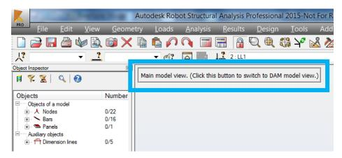
You're currently viewing the Main model view (full stiffness, no notional loads, etc.). Clicking this button will toggle to the DAM model view:
