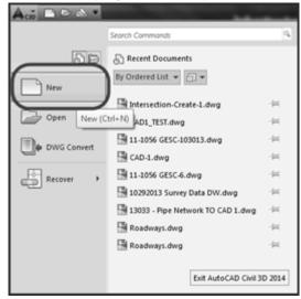
• Use the default imperial template, "\_AutoCAD Civil 3D (Imperial) NCS.dwt" for the new drawing.
