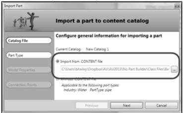
In the Part Type section, fill in the appropriate values. Currently, the only available industry is Water. Make sure your Part Type is chosen correctly as this will put the part in that section when editing the catalog and when adding it to your parts list. If you have added similar parts already, choose the appropriate Part Family Name. If this is the first part you've added for this family, type in the family name and then it will be available for the next part you import.
