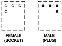
Number and arrangement of pins should agree with actual type of connector used.
