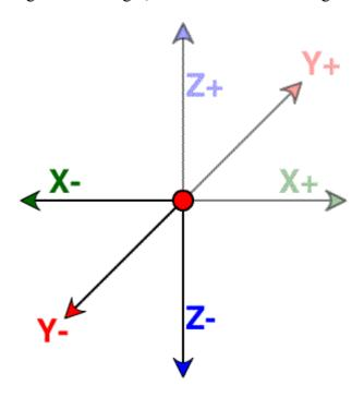
With this system we can therefore indicate any point in a space. For example, to indicate the point on a wooden panel where the machine must make a hole, we will consider that point as the result of intersection between coordinates X, Y and Z.
