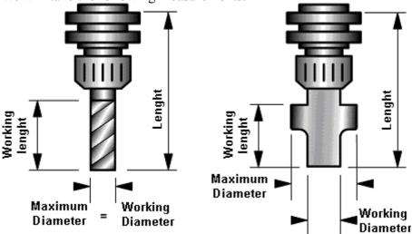
This information will be entered in the tooling file together with other parameters (such as rotation speed, feed-path speed, etc.).
