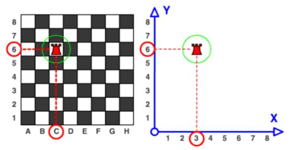
These two coordinates are sufficient to indicate a square on the chessboard. In the case of our bore-milling machine it is necessary to add a third coordinate that indicates the vertical movement along the depth. This third coordinate is indicated as one third of the axis called **Z**. We would therefore have this type of coordinates diagram:
