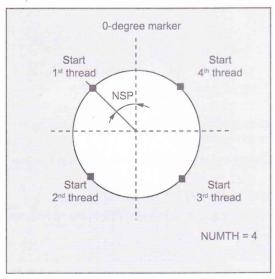
Use the NUMTH parameter to define the number of thread turns with a multiple-turn thread. For a single-turn thread, the parameter must be assigned zero or can be dropped completely in the parameter list.
