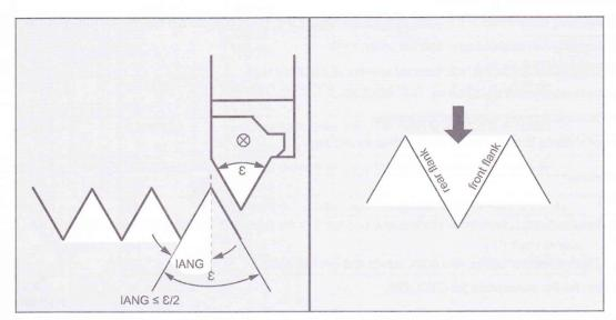
By using parameter IANG, the angle is defined under which the infeed is carried out in the thread. If you wish to infeed at a right angle to the cutting direction in the thread, the value of this parameter must be set to zero. If you wish to infeed along the flanks, the absolute value of this parameter may amount maximally to the half of the flank angle of the tool.
