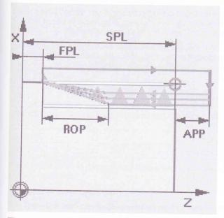
The programmed starting point (SPL) or end point (FPL) constitutes the original starting point of the thread. The starting point used in the cycles, however, is the starting point brought forward by the run-in path APP.
