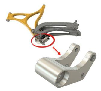
Using 2.5 Axis Functionality, we will begin with a block of <u>Aluminum Stock</u> mounted in a Vise (see Figure 1), and will create three (3) 'job setups' that will be required to machine the Rocker Arm.
