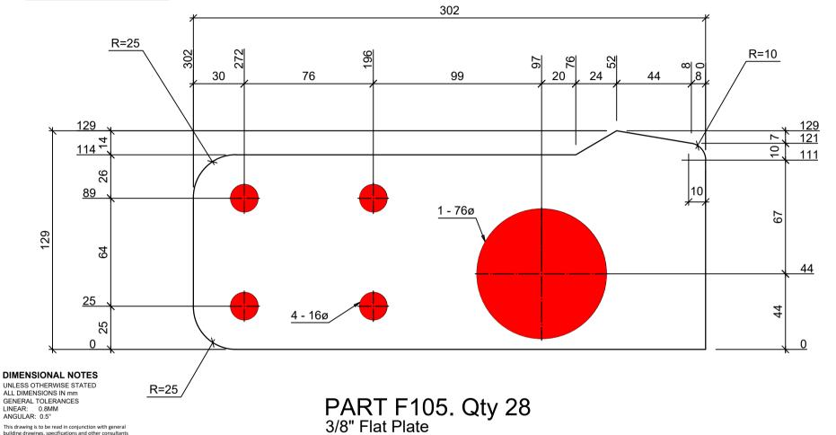
LINEAR: 0.8MM ANGULAR: 0.5° This drawing is to be read in conjunction with general building drawings, specifications and other consultants drawings applicable to this project. All figured
