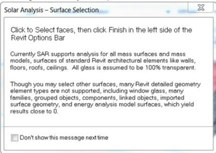
Insight Solar Analysis with Revit does not assume any material properties. Surfaces are assumed to be either completely opaque, or completely transparent. For this reason, it is not advised to conduct solar analysis on transparent surfaces, like glazing or curtain walls for example. This is an important consideration also if you want to look at solar insolation values inside your building (essentially, solar heat gain coefficient (SHGC) impacts will not be represented in results).
