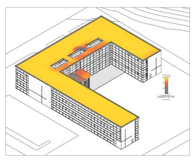
To make any changes to the analysis settings, or select new surfaces for analysis, simply edit the settings or selections, and press **Update** again. New results will override previous results. Note that solar analysis results cannot be saved with the Revit model.
