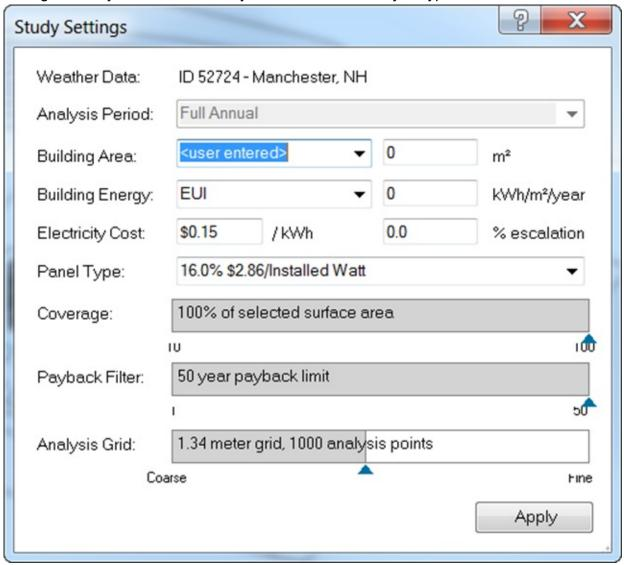
Building area, building energy, electricity cost, and escalation rate can be entered based on energy analysis results from Insight. These values will be used to calculate energy offset predictions and energy costs savings.
