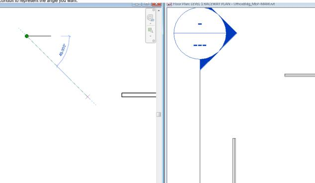
Grab the horizontal conduit and start drawing conduit over to the angled reference plane you just added and then draw it up a short distance along the reference plane. Stop drawing in section view and go back to the plan view. The just use the fillet tool to interconnect them.
