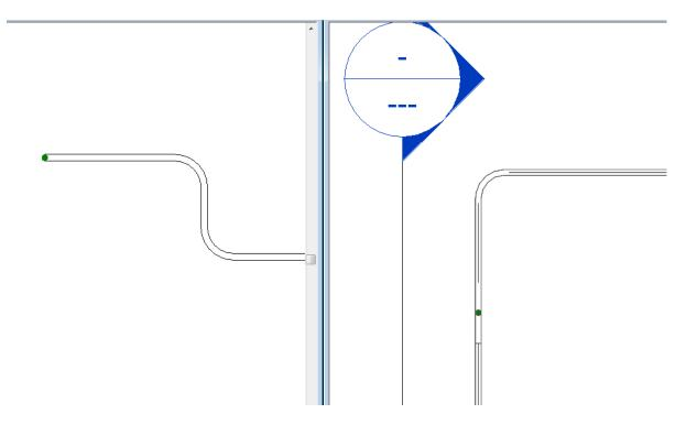
To get the elbow with a kick. Just go to the section view and draw a reference plane from the conduit to represent the angle you want.
