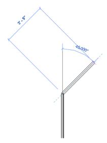
In this next example you often run into a condition where a conduit is drawn in one plane and you are trying to connect it to another conduit drawn on a different axis plane. If you just try cutting a section so you can see both of them and then select one and try to draw a conduit from the end of one to the end of the other, you'll likely get the "no auto-route solution found" error message. That's because Revit seems to like to connect items on the same plane.
