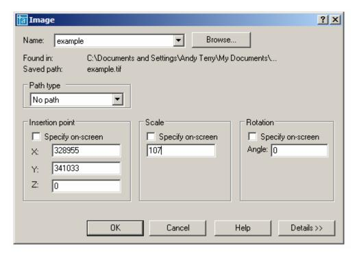
Simply insert the bottom left Easting and Northing as calculated
