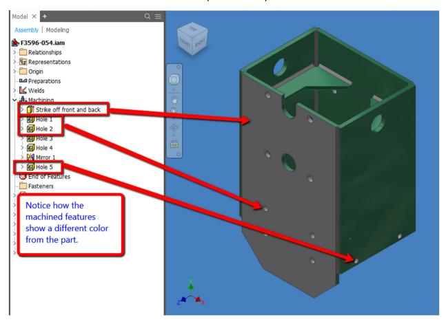
To do this, we first set the color of the part to the "machined" color. Then paint the color of the surfaces to the actual "paint" color of the assembly. Now open one of the individual parts and set the color from the color drop-down. This will be the color of the "machined" surface. I picked "Grey", but it could be any color in your library.
