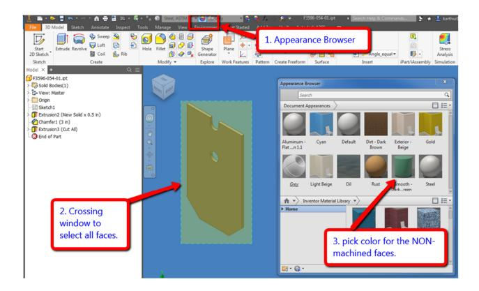
Next return to your Weldment assembly. You may have to update the model. You should nowyou're your model with all the machined features a different color from the "non-machined" surfaces.
