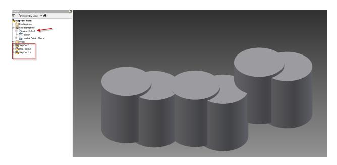
Here's my top assembly. I inserted my sub-assembly 3X .. All components are shown at this level.
