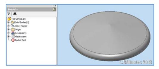
Save the file into your directory, and let's create the flat pattern model using Derive tool located in 3D Model tab, Create Panel. Create New file, use Standard(mm).ipt and now click Derive tool and direct the file to part that has just saved. Turn off Solid Bodies and turn on Sketches then click OK button.
