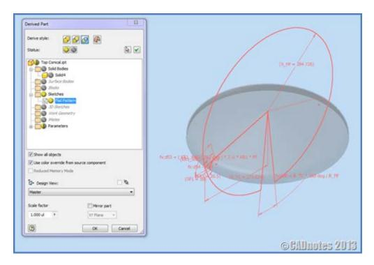
And the last is to extrude the sketch. Try to change the dimension of Top Conical, and see that any changes in your flat pattern file will also update the model.
