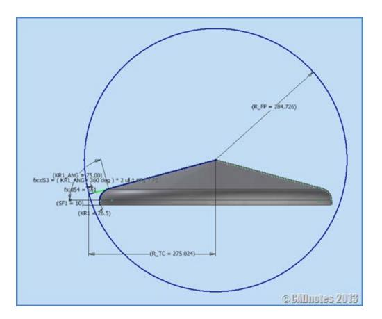
Let's create apex angle by adding line from the center of circle. Add horizontal constraint in the end of line that touches the arc of circle. Add the equation as you can see in the picture. Let's calculate the equation using calculator:
