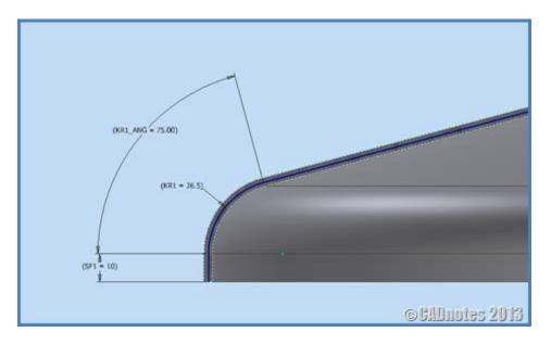
Add two segment of line to define the outside dimension of sheet metal that have to be prepared as raw material. To make your flat pattern update as far as there is a change of Top Conical dimension, let's make the equation for the line as shown figure below.
