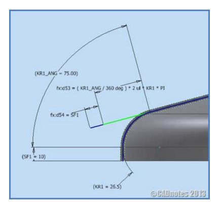
Next step is to create the circle as flat pattern of this Top Conical part. Add one more reference dimension. Same with before, this reference dimension is used to create apex angle equation of this flat pattern. To create this flat pattern sketch, we need to define the apex angle.
