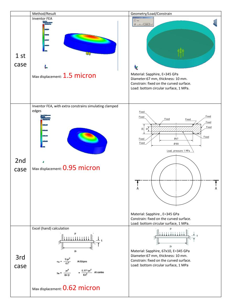
Simple loaded circular plate supported by clamped edges
