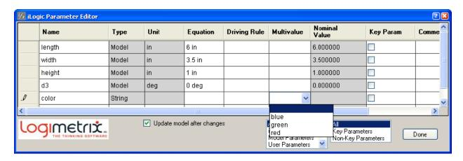
We will construct a rule that will modify the color of the model based on the value chosen for the parameter called color. This will be done with a series of if/then statements.
