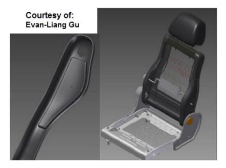
Use freeform along with parametric modeling to create a more visually compelling design.
