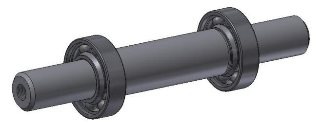
For this example, we will heat up the bearings, and cool the shaft down to achieve our press fit.
