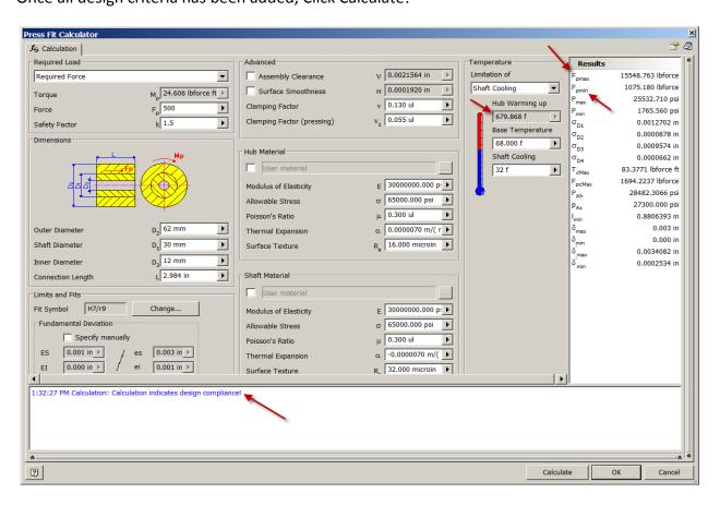
We see our design is within compliance, also, we can read what our max/min force needed to drive the bearing up to the journal seat! Also, what temp our bearing should be heated too.
