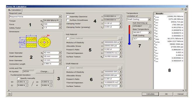
Section 1, Required Load: We are looking for the Required Force. Other option would be to Calculate for required torque. Basic Force to Start will be 500lbs.
