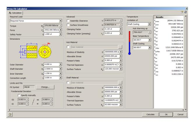
In the following example, we will use a 10" lg. steel shaft, 30mm Dia., with a 12mm bore running the entire length. 2 AFBMA 30X62x18 bearing will be press on from both journal ends. We will calculate the Force required to press the bearing on to they hit the journal end:
