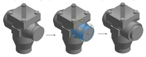
Recognize extrude Recognize extrude features, and convert them to extrusions recognized by Revit.
