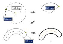
center arc, and by slot width.
