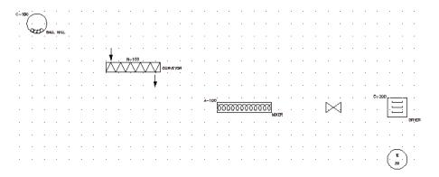
**TIP** Align the components horizontally and vertically using the Align tool to make inserting the pipes easier.
