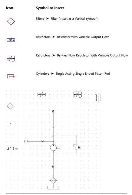
**TIP** Align the components horizontally and vertically using the Align tool to make inserting the pipes easier.
