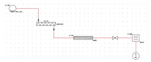
**4** In the AutoCAD Layers toolbar, change the wire layer to POS and the linetype to HIDDEN2.
