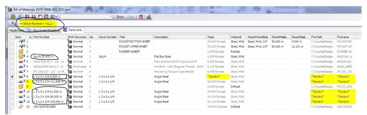
If you were inserting this entire light board frame assembly into a parent assembly and wanted it to appear as a single item in the parent, simply make this assembly inseparable in the parent assembly and it will appear as a single line in that drawing parts list. (There is one caveat with this though - purchased items will propagate up. That is typically why I change most of my CC hardware to "Normal". In this case, the hex bolt will also show up in that new parent assembly.)
