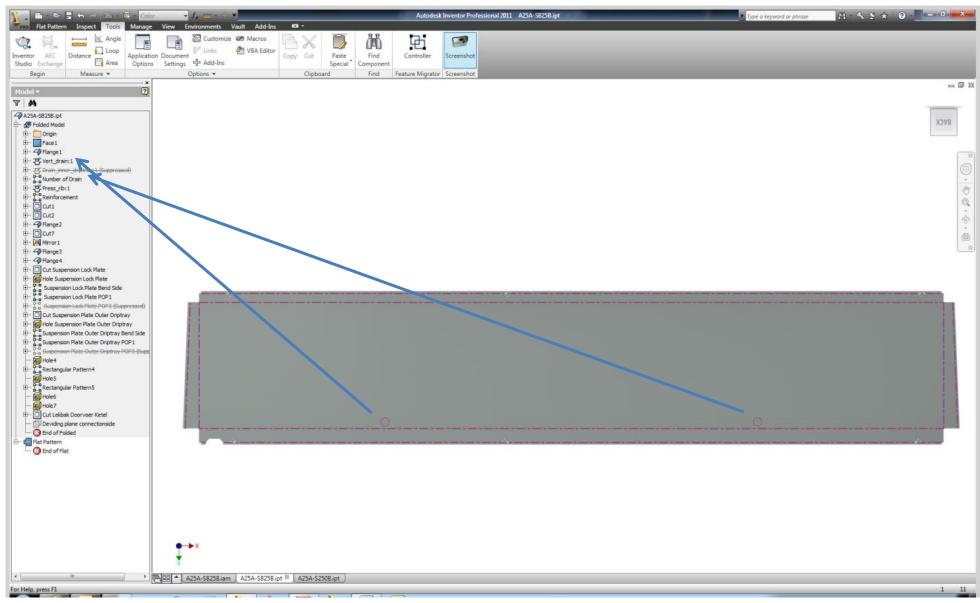
We have in the model part a punch (vert\_drain) with a simplified sketch. When we look at the flat pattern of the model part, the simplified sketch is shown correct.
