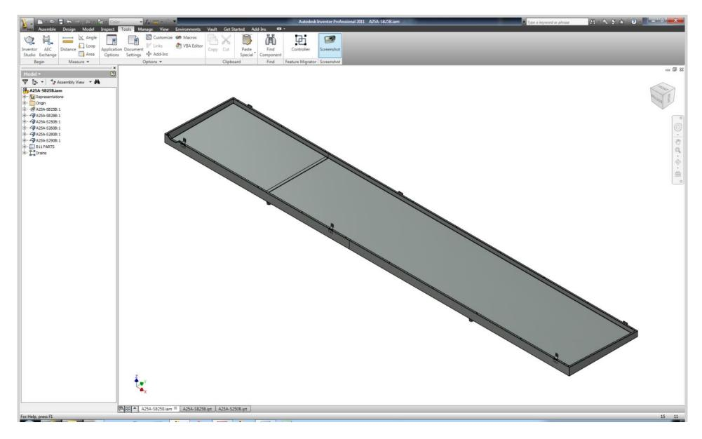
We use BaseOuterDripTray2Sections as model part to apply all changes. Parts A25A-S250B and A25A-S260B are divided parts of the derived component of the base model.
