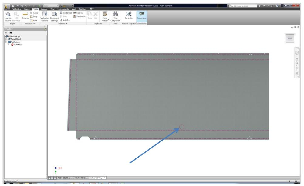
When I place a new punch in the model part, and update the derived part, the simplified sketch of this punch is correct. When I remove the pattern of the first vert\_drain punch, and remove the dimension in x-direction (1014mm) and then update the derived part the simplified sketch is also shown correct. But when I place again the x dimension or a pattern, the simplified sketch is showed mirrored again. What could this be, and how can I solve it?
