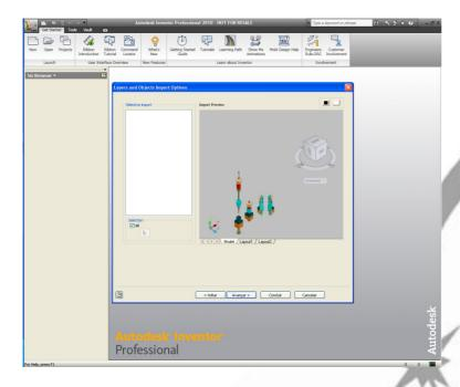
In "Import Destination Folder" select **3D models** in the **3D solid options** and select **New part > Wires to 3D sketch** in the **Destination for 2D data** area. (You should specify the unit). Click **Done**
