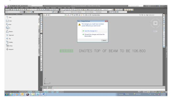
Step 3 after saving the block it will go to Layout mode instead of staying at model mode.
