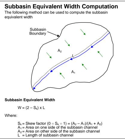
Figure 9.4 Method for computing an equivalent subbasin width for determining the time of concentration (Tc) for some Tc methods
