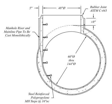
Pipe Manufactured To ASTM C-76 Specifications, Reinforcing Class As Required.
