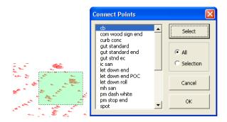
Select one or more of the descriptions in the list and hit OK. A separate 3d polyline for each of the codes will be drawn connecting the points in order of point number.
