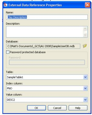
Do the same for the elevation. Except that you will need to create a new connection with a different value column.
