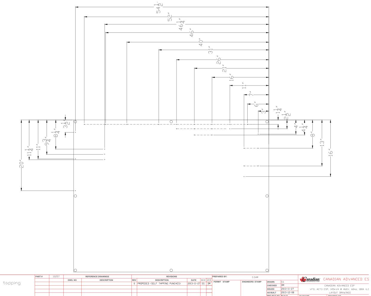
1. 10-16 X 3/4 is the size of self tapping screw. P/N is 5000-0850-060B
