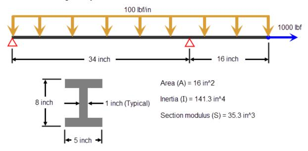
**Find**: The bending moment and axial force within the beam using a 3-D brick model.
