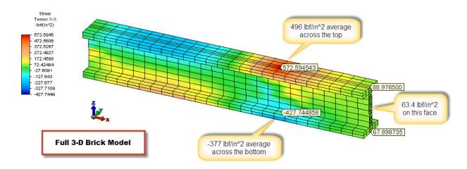
The differences between the real world and the simplified hand calculations are trade-offs that engineers have been dealing with for a long time. For this exercise, let's use the average stresses across the width. Using the two equations above and entering the values gives<sup>5</sup>:
