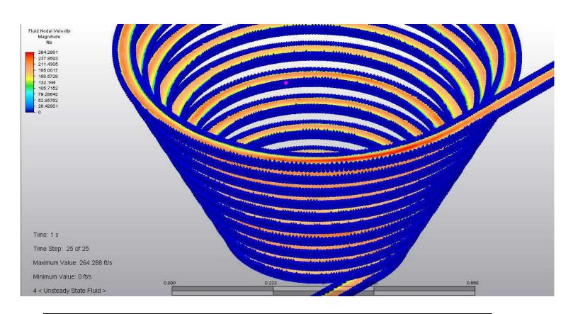
Unsteady state. 58% Tet mesh, automatic refinement points. 0.003 Velocity and Pressure Norm. Perform max iterations. Convergence tolerance 0.01. This looks good!
