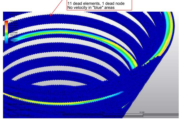
With 0.4 ID, 0.5 OD Tube (tube turned off during fluid analysis)
