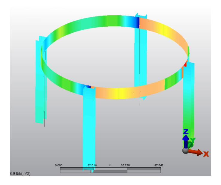
Is the resulting moment created by the beam offset considered in this evaluation. As I understand the explanation in the Help section, the analysis considers a solid plate joint between the connecting members. Does this plate section add rigidity to to that joint? In the case being considered, does the connecting plate end at the at the bottom of the steel ring and therefore allow the resulting moment to transfer into the lower leg evaluation:
