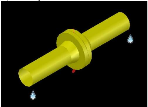
Properties Flange: flange thickness is: 23.876 mm
