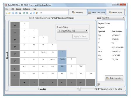
**Branch Fitting** Sets the current fitting type or stub-in. Setting a value does not update the selected branch table cells immediately. To apply the current fitting type, click Apply to Table.
