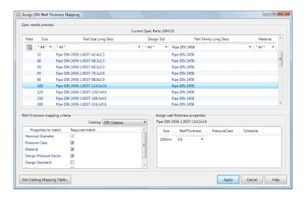
**Spec Results Preview** Displays parts in the current spec sheet. You can select a part to assign its wall thickness.
