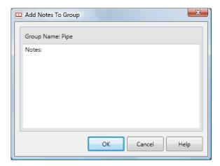
**Group Name** Specifies the name of the spec sheet group. The note is set for the entire group. Notes are included when the spec sheet is printed.
