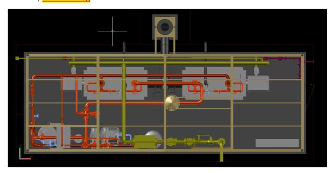
2) I make new file: ortho.dwg and insert XREF - MODEL.dwg. Xref was made like attachment. And turn off some layers in ortho.dwg.
