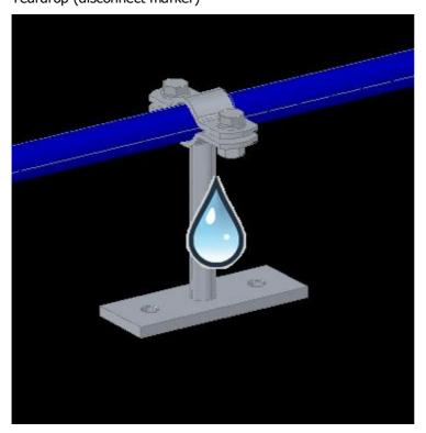
For example: Simple Pipe Support from TOOLPALETTE : Is oke.
