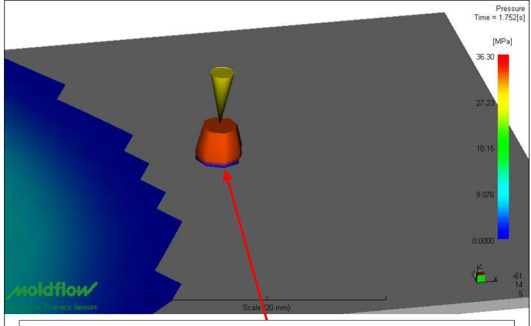
Because, in the beginning the injection process (when the gate 2 is close), the pressure is high in the runner and in a part of the gate but not in the last element of gate.
