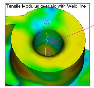
No variation in mechanical properties (Tensile modulus) is observed along the weld line region ?
