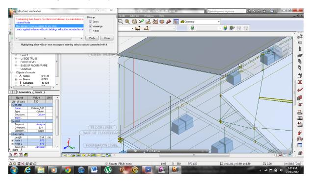
The element above has not been assigned to a storey and that is the properties for it
