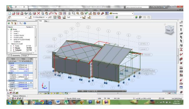
This is the elements that is defined outside the geometric limits of the assigned story (after I assigned it to level 1)
