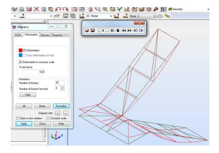
Deflection pattern moves up and down between initial position and deflected structure as illustrated
