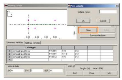
Correctly set your first vehicle with the definition table. For the example, a symmetric vehicle has been created.
