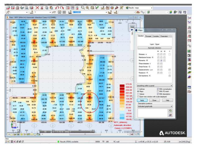
Moment to be used for designing the tension reinforcement in X-direction:
