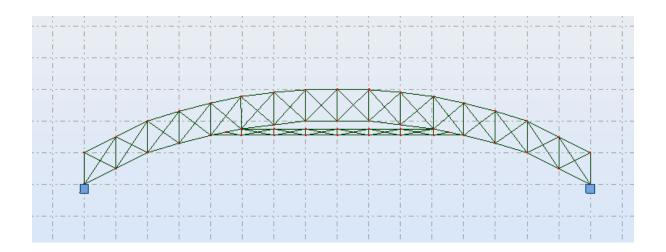
This is what I have designed. it is to be an 80m span roof truss. To be made out of steel.
