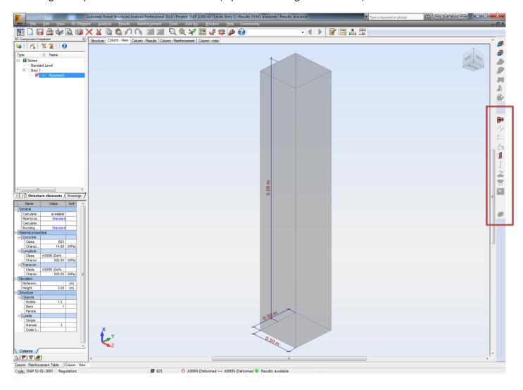
Column results are given according to A500 reinforcement by default and for zero bending moment value!
