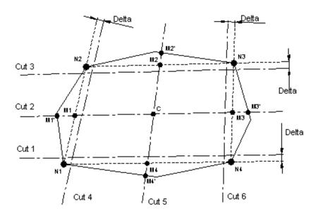
In order for cross-sections 1, 3, 4 and 6 to be correctly defined within panels (no defined coordinates), move the cross-sections by the Delta value with respect to the main panel nodes N1, N2, N3 and N3. The delta value equals the tolerance value applied in the generation of the calculation model.
