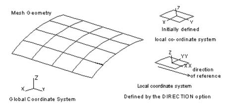
The following define the sign convention applied to forces for planar finite elements.
